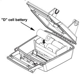
Install batteries in power case battery adapter.
